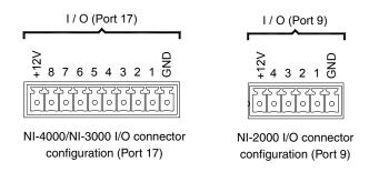
FIG. 15 INPUT/OUTPUT connector (male)
